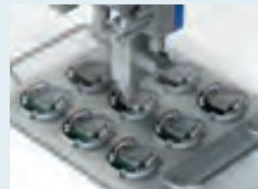
Potting onto small components.
