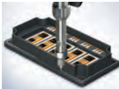
CIPG seal dispensing on IGBT modules
