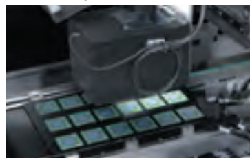
Dispensing inspection machine
