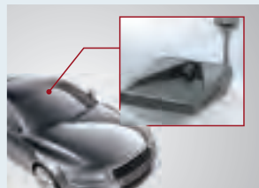
ADAS holder bonded to windshield
