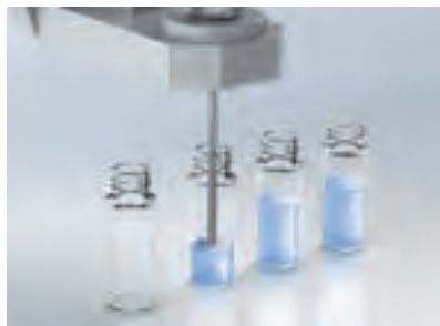
Dispensing reagents into vial bottles
